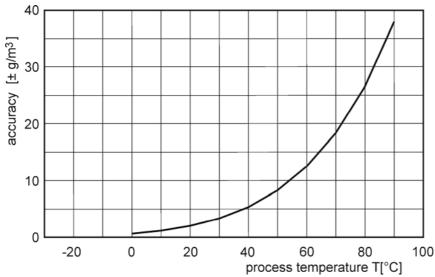
Accuracy and range of computed dew point temperature for compressed air measurement up to 25 bars.
