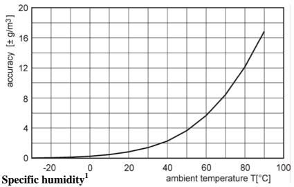
Accuracy:  $\pm 2g/kg$  at ambient temperature T < 35°C (95 °F)
